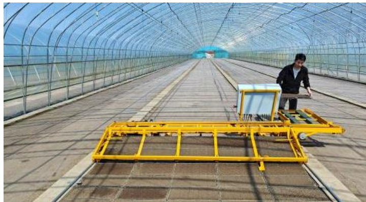
Fig. 11 – Field test of the seedling tray placement machine
