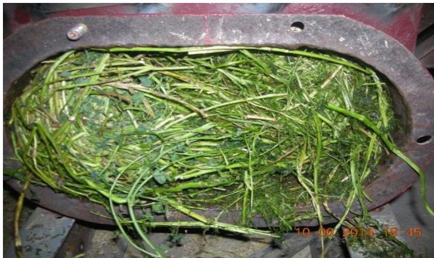
Fig. 2 - Compaction of the twisted mass as it passes through the diffuser
