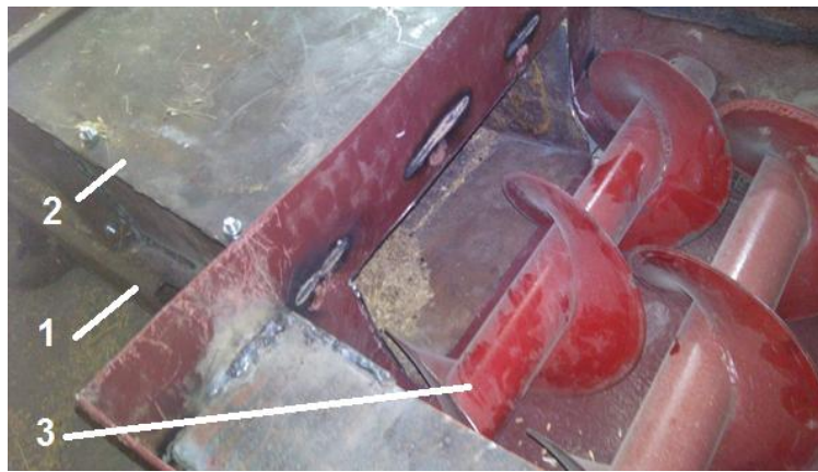
Fig. 1 - Equipment for plant raw materials compaction 1 – frame; 2 – feeder; 3 - twin-screw compactor.
