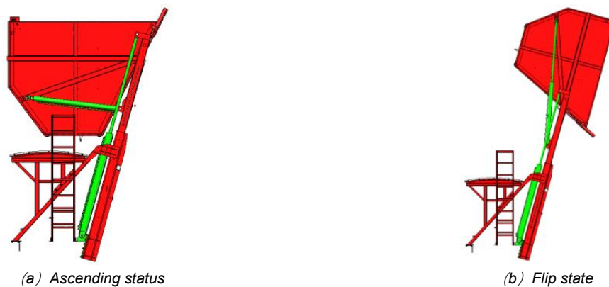
Fig. 12 – Operating status of grain collection box
