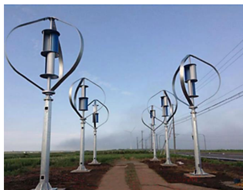
Fig. 26 - Combination of Darrieus and Savonius wind turbines
