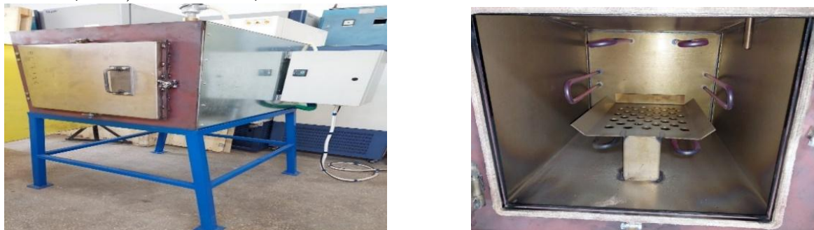
Fig. 4 - Equipment for biochar production to enhance soil moisture retention
