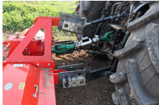
(b) Torque sensor installation diagram
