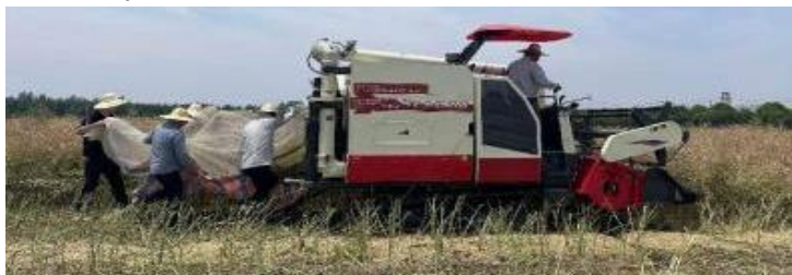
Fig. 8 - Field Performance Test of the Rapeseed Single Longitudinal Axial Flow Full-Periphery Separation Harvester
