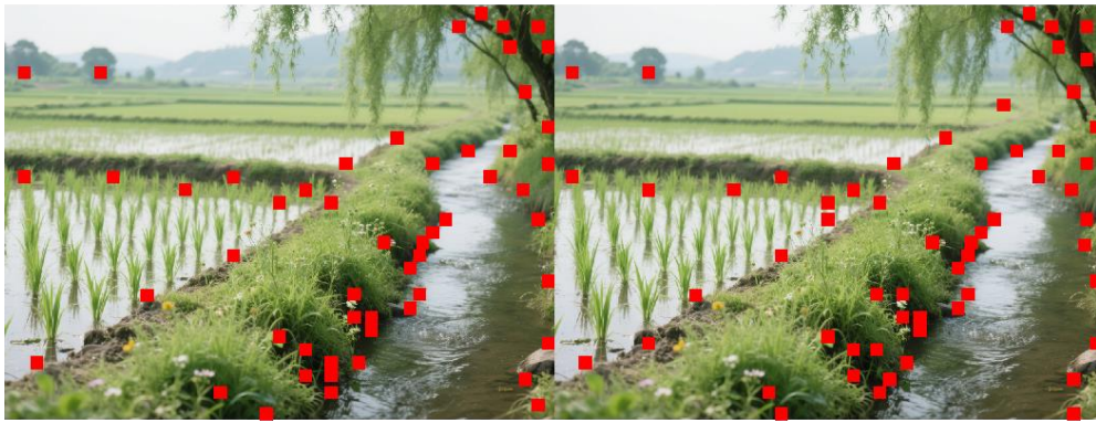
Fig. 3 - ORB feature point extraction results
