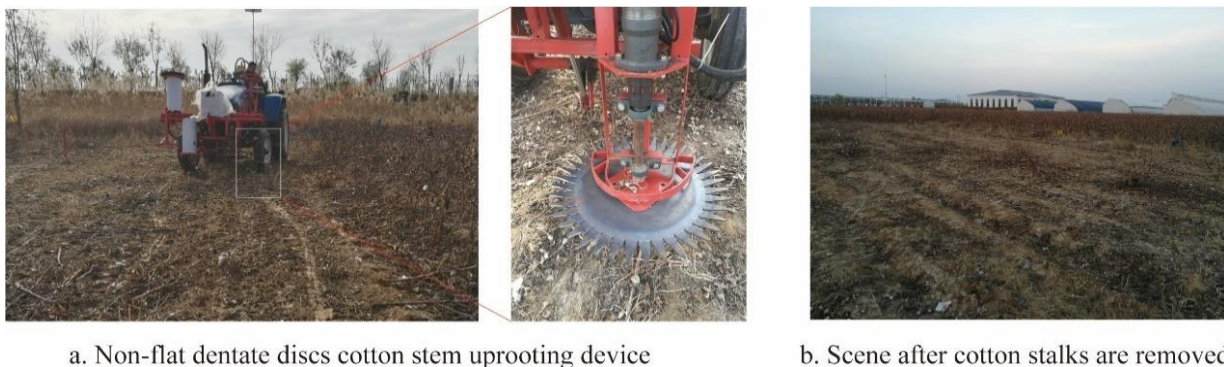
Fig. 10 - Cotton stalk removal test
