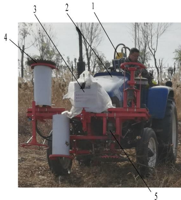
Fig. 2 - Toothed disc multi-row cotton-stalk uprooting device
