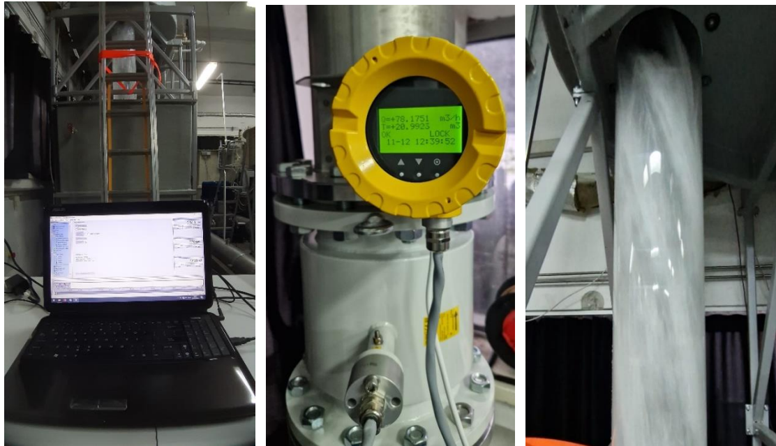
Fig. 8 – Testing of the integrated low head micro-hydro turbine
