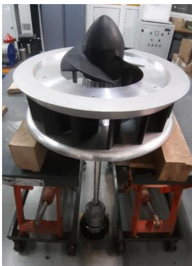
Fig. 4 – Low head micro-hydro turbine assembly ready for testing
