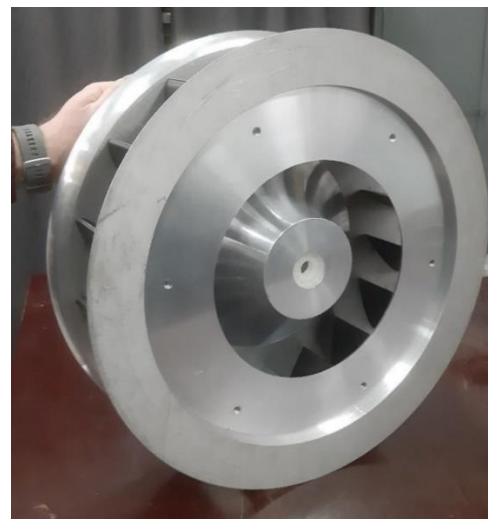
Fig. 4 – Low head micro-hydro turbine assembly ready for testing
