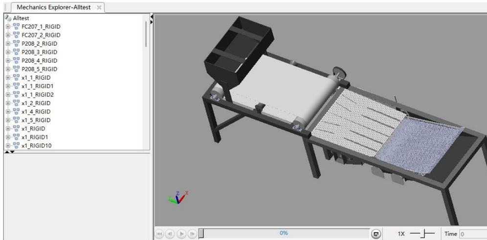
Fig. 7 - The mechanical operation diagram generated by Simscape
