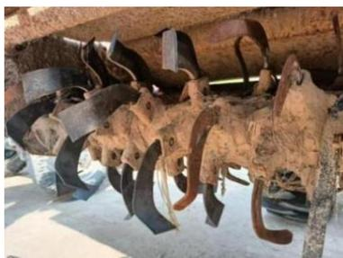
**Fig. 14 - Schematic diagram of rotary tilling blades installation**
