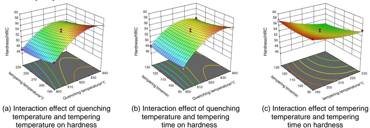
Fig. 11 - The effects of the interaction of various factors on the hardness of rotary tilling blades
