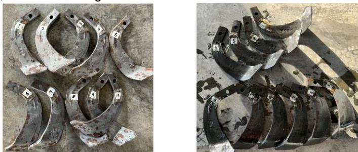
(a) Unquenched rotary tilling blades (b) Quenched rotary tilling blades
