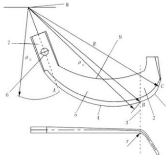
**Fig. 5 - Schematic diagram of the structure of the rotary tilling blades**
