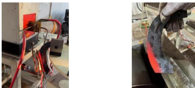
(a) Test site (b) Quenched samples
