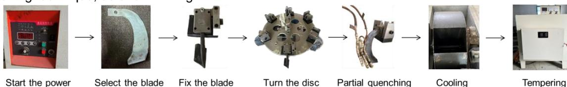
Fig. 1 - Flow chart of high-frequency partial quenching technique of rotary tilling blades
