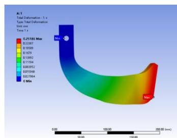
Fig. 9 - Total deformation contour diagram
