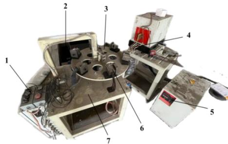
**Fig. 4 - Rotary tilling blades high-frequency partial quenching device**
