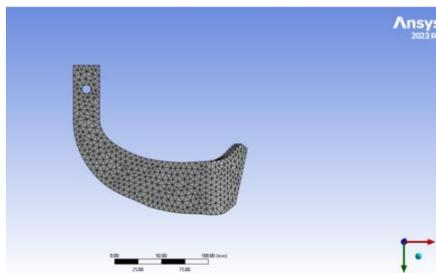
Fig. 7 - Meshing the model
