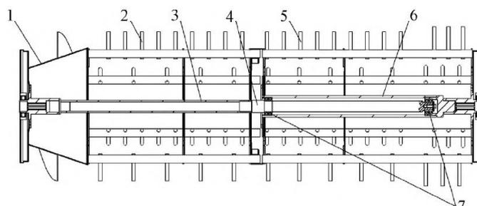
**Fig. 6 - Structure diagram of differential threshing cylinder** (Kang et al., 2023)
