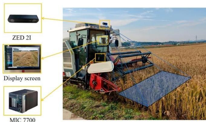
Fig. 11 - Visual data acquisition system for feed quantity (Zhang et al., 2024)
