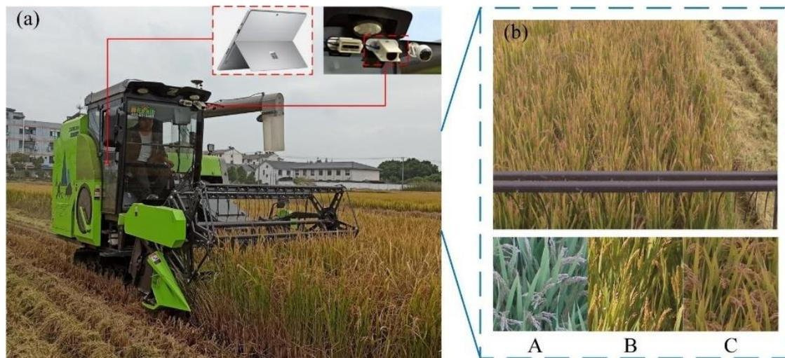
**Fig. 12 - Real-time rice spike density detection image acquisition** (Sun *et al.*, 2024)
