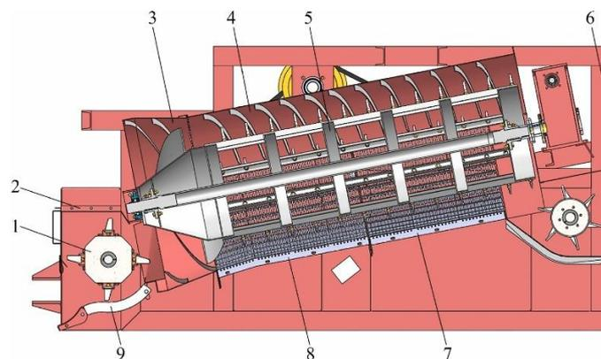
**Fig. 5 - Tangential and longitudinal-axial threshing and separating unit (Yuan *et al.*, 2024)**
