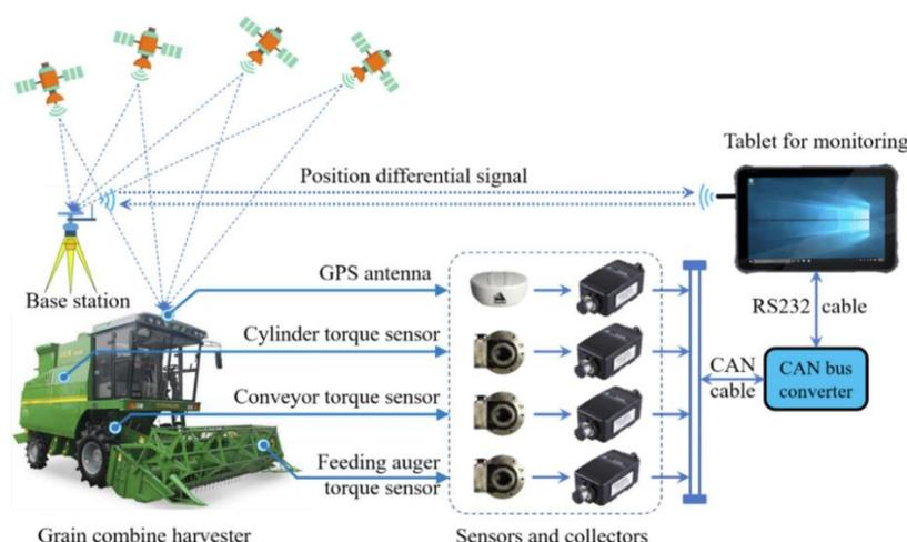
**Fig. 9 - Multi-sensor fusion-based crop feed rate detection method** (*Zhang et al., 2022*)
