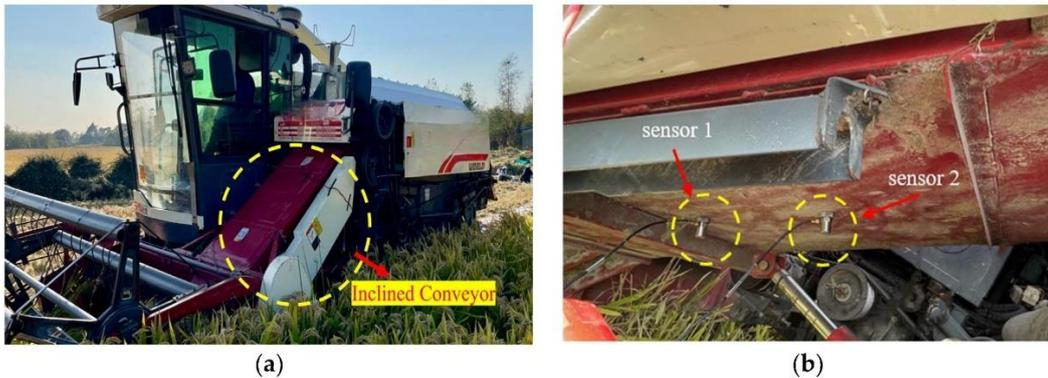
**Fig. 8 - Installation positions of the vibration acceleration sensor** (*Abdeen et al., 2022*)
