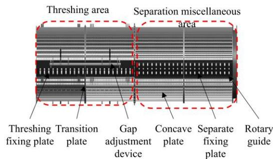
Fig. 2 - Schematic of rotary concave screen (Tang et al., 2024)
