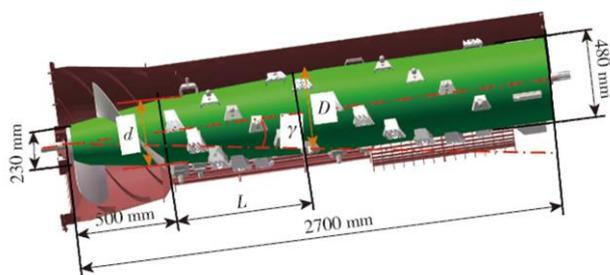
Fig. 1 - Variable diameter threshing drums (Wang et al., 2021)
