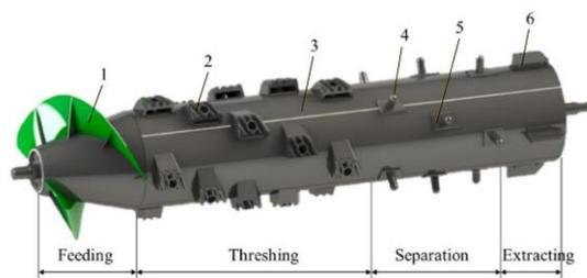
1.Screw feeder; 2.Rasp bar threshing element; 3.Drum body; 4.Rod-tooth threshing element; 5.Installation base; 6.Exclusion board
