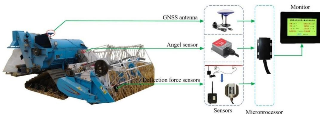
Fig. 10 - Design of the feed rate monitoring system (Chen et al., 2025)
