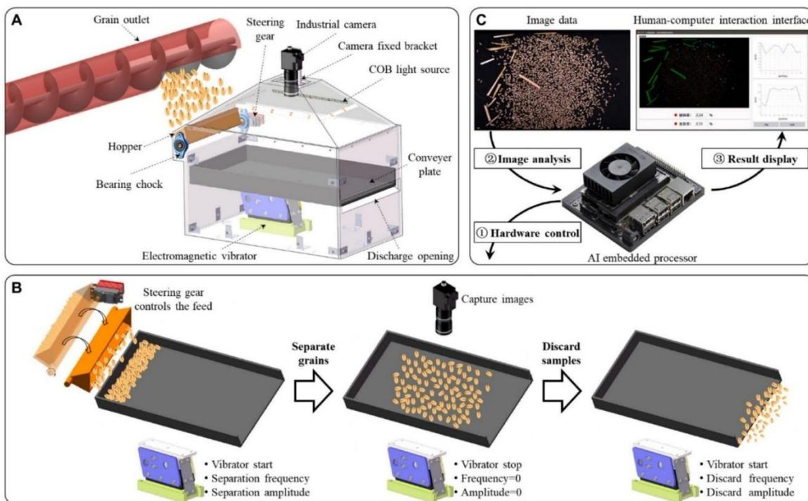
Fig. 14 - Wheat broken rate and impurity rate detection system (Qi et al., 2024)
