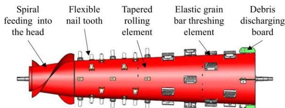
Fig. 3 - Flexible nail tooth and elastic grain bar threshing drum (Song et al., 2022)
