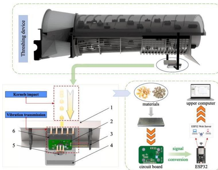
**Fig. 17 - Structure and signal processing workflow of the entrainment loss monitoring sensor (Dong *et al.*, 2024)**
