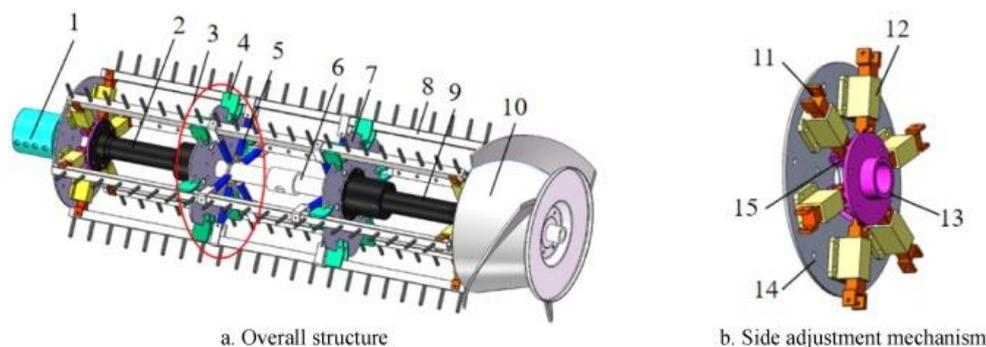
**Fig. 7 - Schematic diagram of the variable-diameter threshing drum**
