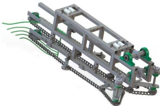
Fig. 1 – 3D Conveying and tipping device test platform model
