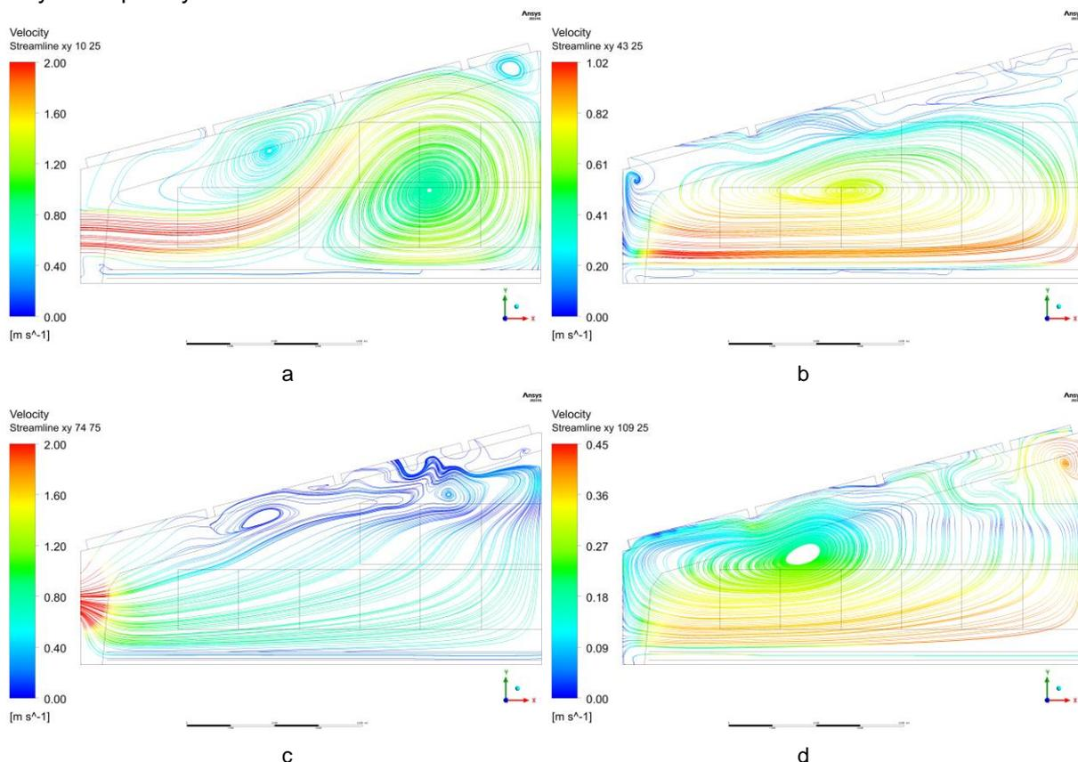
**Fig. 2 - The air flow lines ( $\text{m}\cdot\text{s}^{-1}$ ) in the poultry house along the xy axis at different distances from the front end wall**
