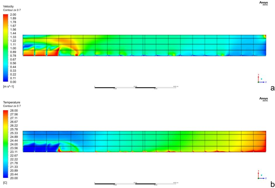
Fig. 4 - The air velocity field, m·s<sup>-1</sup> (a), and temperature field, °C (b), in the poultry house along the zx axis at a height of 0.7 m from the floor level
