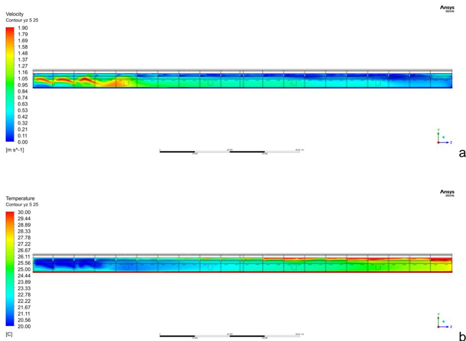
**Fig. 6 - The air velocity field, m·s<sup>-1</sup> (a), and temperature field, °C (b), in the poultry house along the zy axis at 5.25 m from the side wall**
