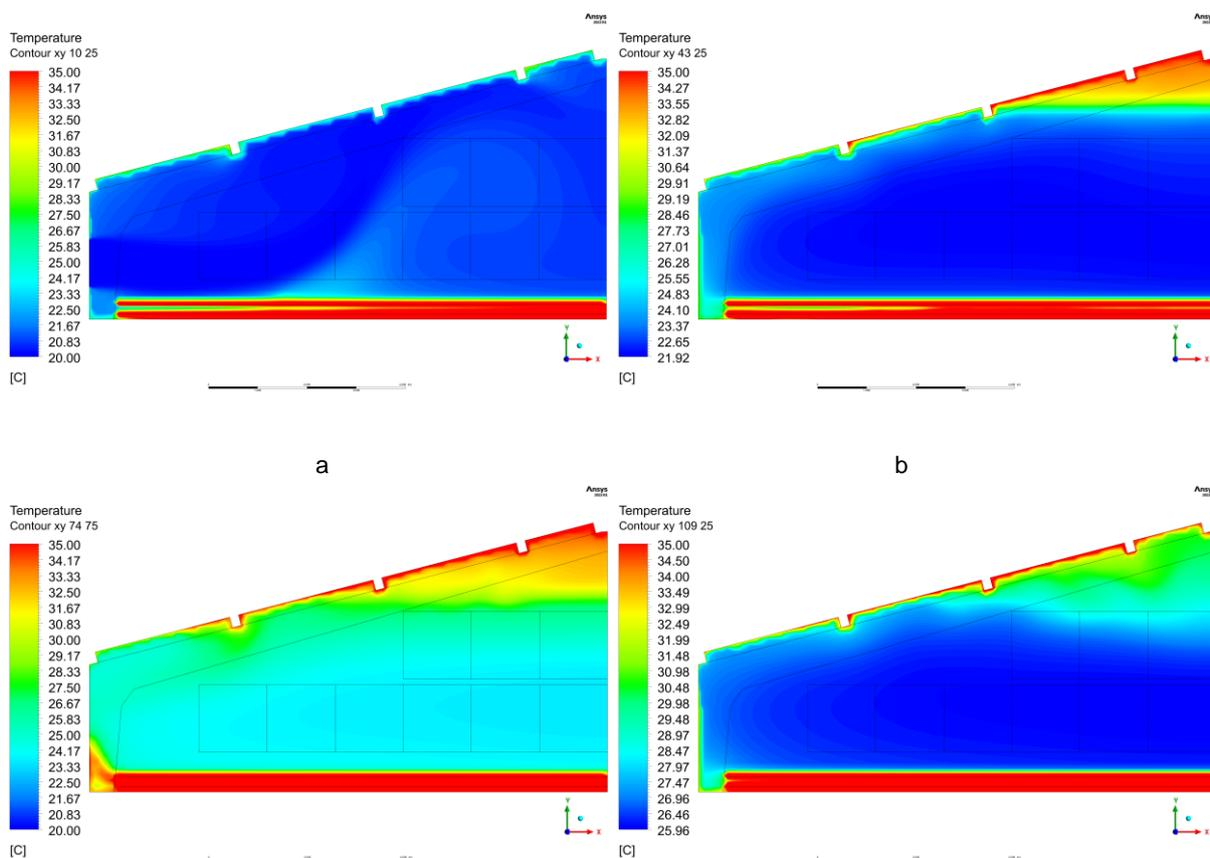
**Fig. 3 - The air temperature field ( $^\circ\text{C}$ ) in the poultry house along the xy axis at different distances from the front end wall**
