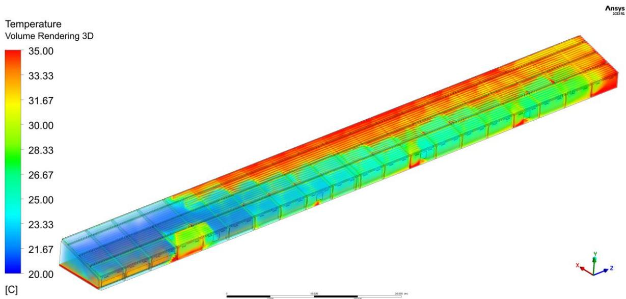
Fig. 5 - The visualization of the air temperature in the poultry house ranges from 20°C to 35°C
