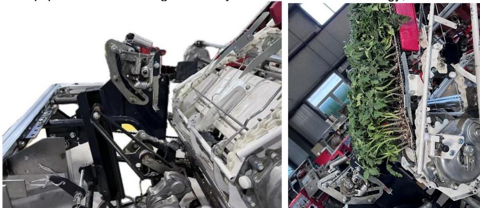
Fig. 6 – Automatic Seedling Picking Device Laboratory
