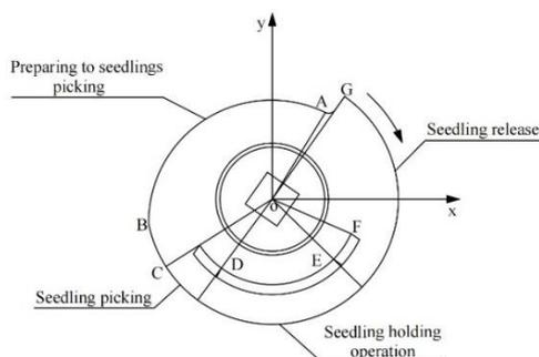
Fig. 2 – Cam working stroke
