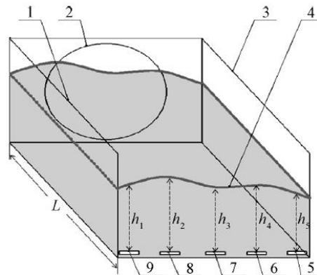
**Fig. 7 - Schematic diagram of particle flow mass flow detected by piezoelectric sensor** (*Xiong et al., 2018*)
