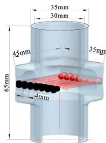
**Fig. 4 - Mass flow detection method of continuous dense particle flow based on infrared sensor**
