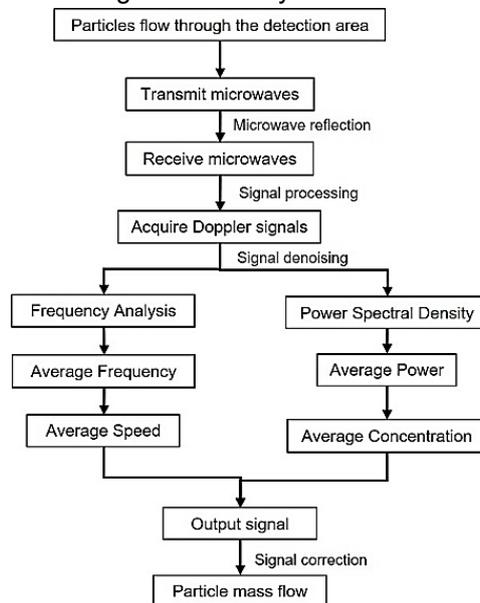
Fig. 8 - Microwave detection method based on doppler effect
