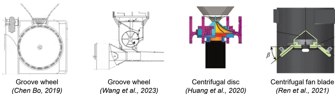
Fig. 10 - Method of displacement regulation and detection for UAV seeding
