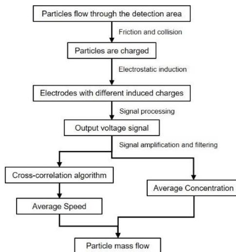
Fig. 3 - Electrostatic method
