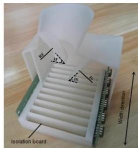
**Fig. 5 - The dense particle flow is divided into a single row of small particle flow** (Liu *et al.*, 2019)
