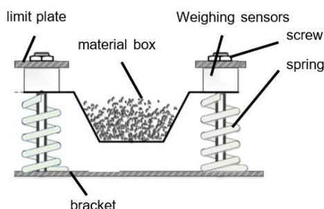
Fig. 1 - Weighing method based on pressure sensor
