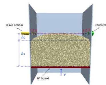
**Fig. 6 - Photoelectric sensor array** (Yin *et al.*, 2021)
