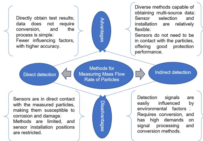
Fig. 9 - Comparison of different detection methods
