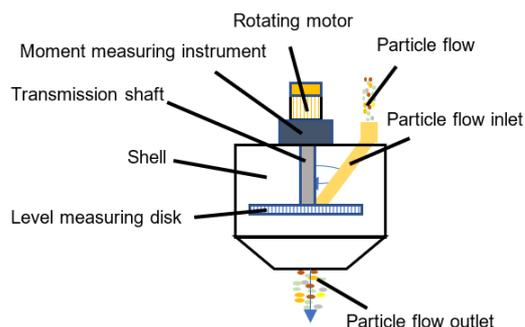
Fig. 2 - Coriolis force method based on rotation mode
