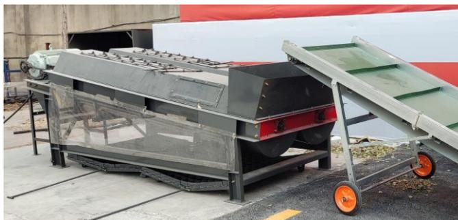
Fig. 7 - Testbed for double longitudinal axial flow with a large feeding amount
