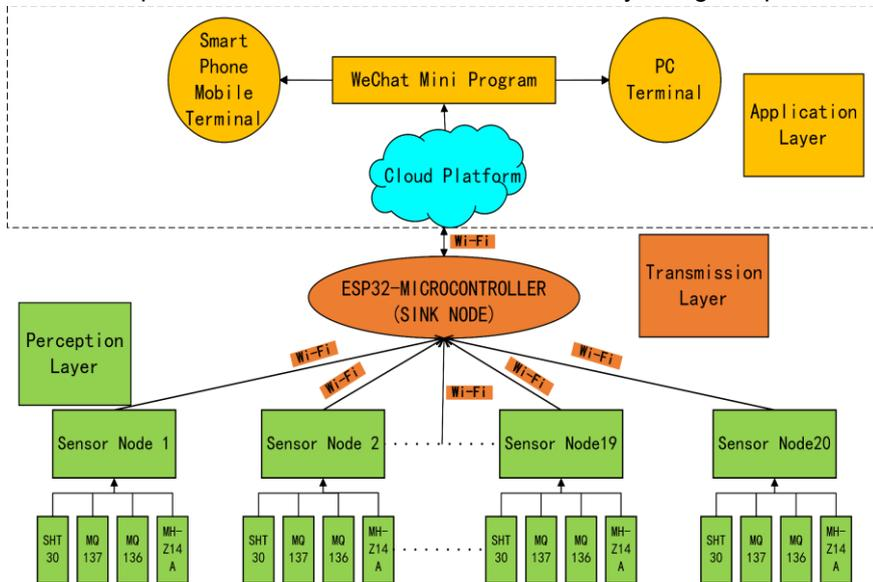
Fig. 2 – Overall system structure
