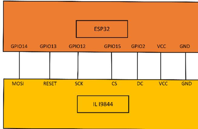
Fig. 4 – Schematic diagram of ESP32 MCU and ILI9488 display
