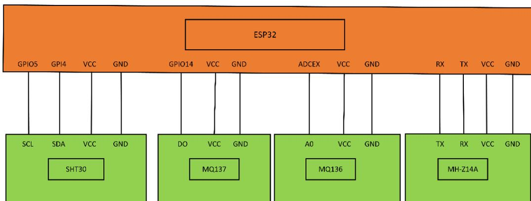
Fig. 3 – Interface between ESP32 and sensor
