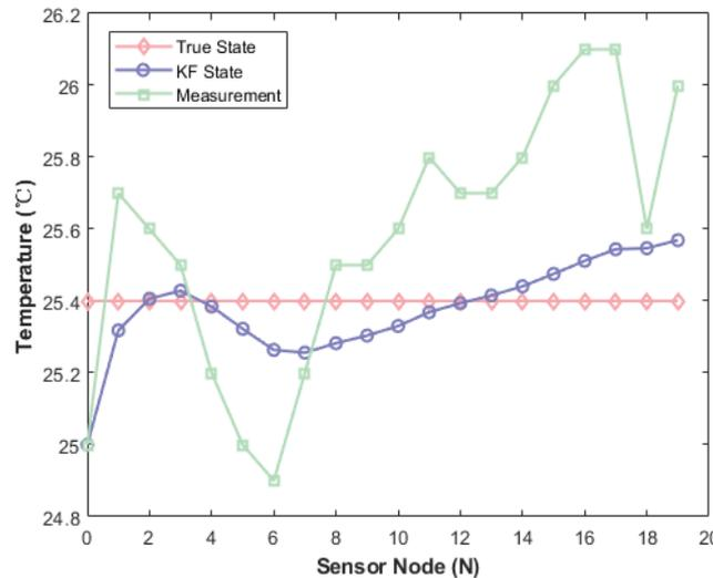
Fig. 6 – Comparison picture of the temperature values measured by three temperature measurement methods
