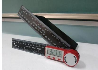
Fig.4(b) - Test rig for coefficient of static friction between PR and PLA plates
