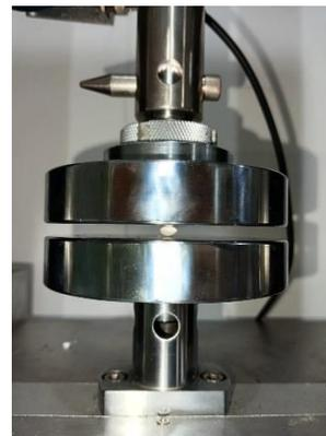
Fig.3 - Pressure deformation test of PR
