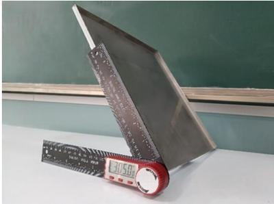
Fig.4(a) - Test rig for coefficient of static friction between PR and steel plate
