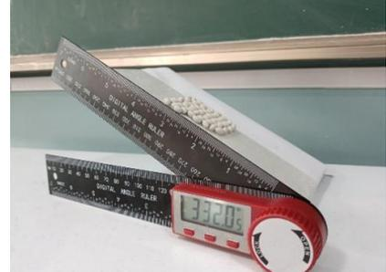
Fig. 4(c) - Test rig for inter-seed static friction coefficient of PR
