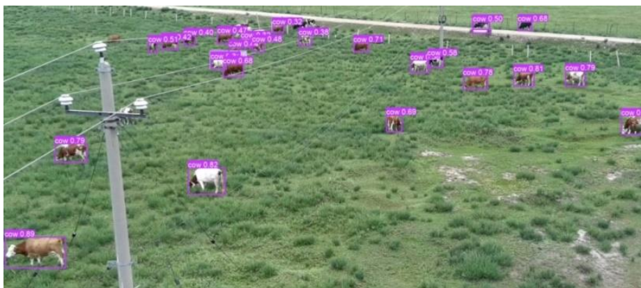
Fig. 2 - High accuracy of YOLOv8 pre-trained on the COCO dataset in detecting cattle during the summer
