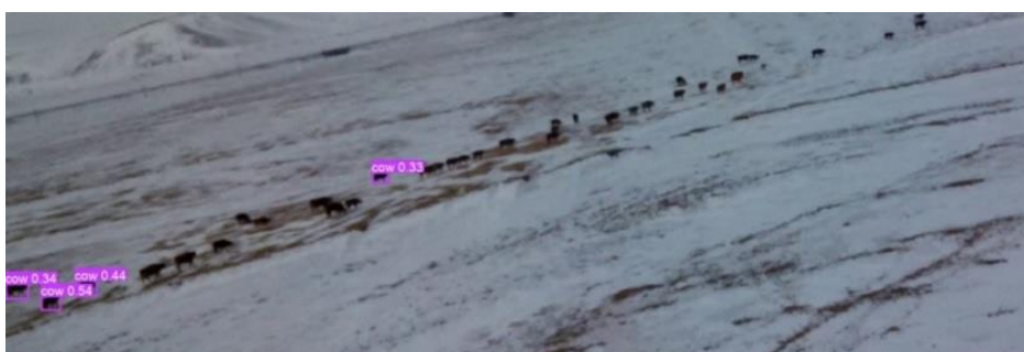
Fig. 3 - Low accuracy of YOLOv8 pre-trained on the COCO dataset in detecting cattle during the winter
