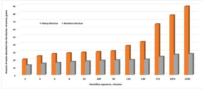
Fig. 7 - Water storage potential in biochar depending on water soaking time
