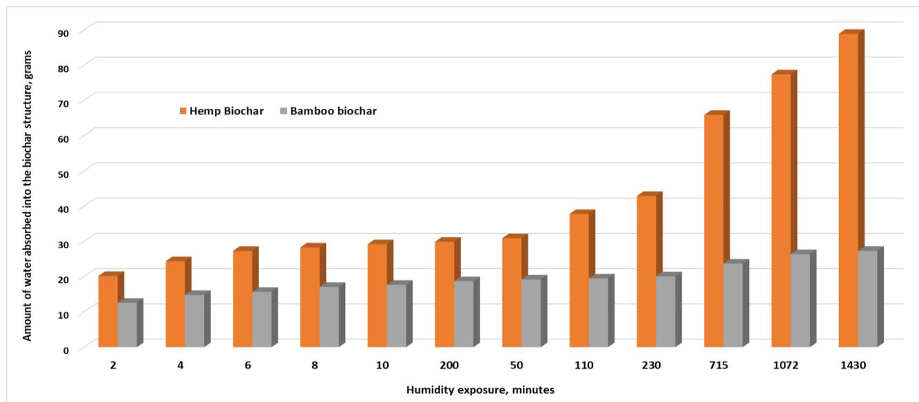
Fig. 7 - Water storage potential in biochar depending on water soaking time
