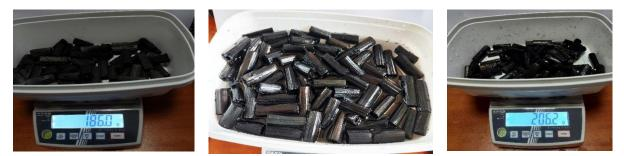
Fig. 5 - Different phases during the experiments to evaluate the water storage potential in biochar
