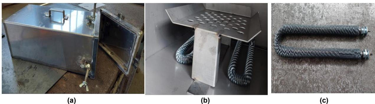
**Fig. 2 - Heat treatment of organic material using a retort and electrical resistance**
