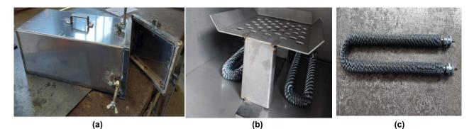
Fig. 2 - Heat treatment of organic material using a retort and electrical resistance a) retort; b) retort support; c) electric resistances
