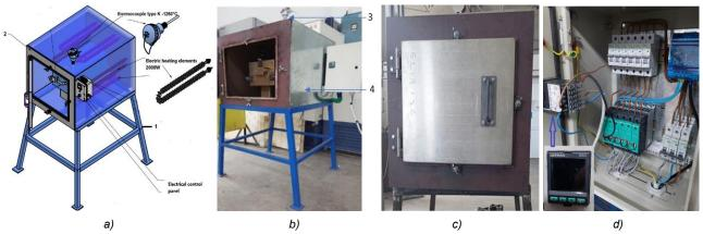
Fig. 1 – Experimental model for biochar production-general assembly a) experimental model for biochar production; b) retort; c) equipment case; d) electrical control panel
