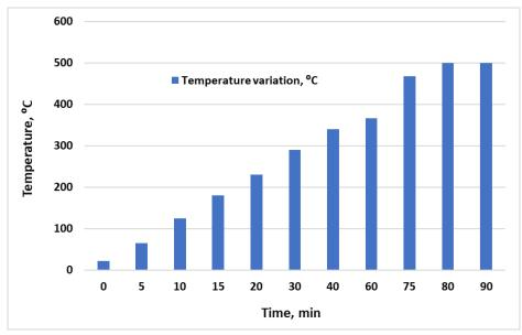
Fig. 6 - Temperature variation over time during pyrolysis equipment operation
