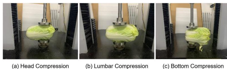
Fig. 4 - Static load compression mechanical characterization of Chinese cabbage plants
