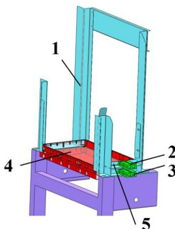
**Fig. 3 - Horizontal tray delivery device**
