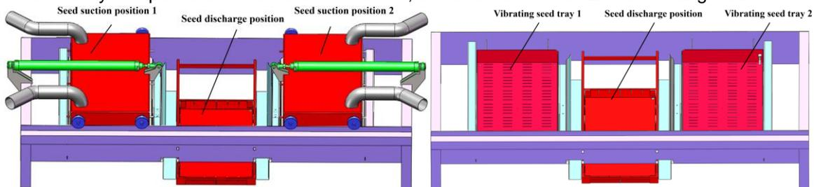
**Fig. 6 - Structure diagram of the dual-station high-efficiency seeding device**
