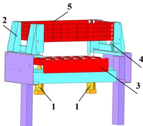
**Fig. 4 - Horizontal tray stacking device**
