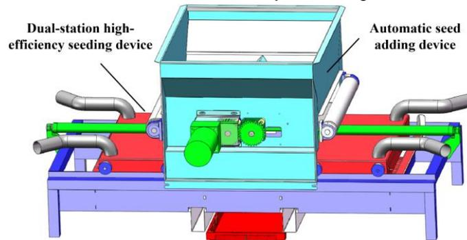
**Fig. 5 - Dual-station high-efficiency seeding device and automatic seed adding device**
