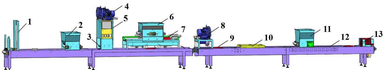
**Fig.1 - Schematic diagram of the overall structure of the whole tray air-suction seeding assembly line for rice precision seedling cultivation**
