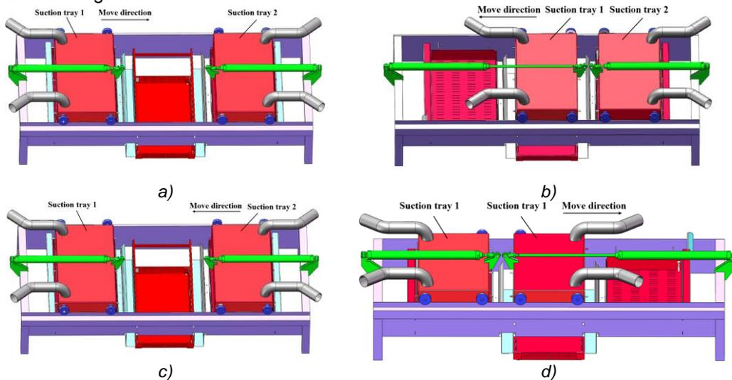
**Fig. 8 - Working principle diagram of dual-station high efficiency seeding**
