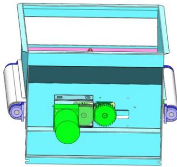
Fig. 10 - Automatic seed adding device
