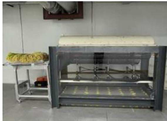
Fig. 8 – Test bench of segmented adjustable threshing device for rice harvesting
