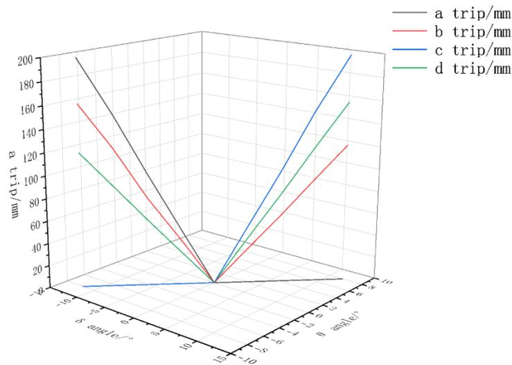
Fig. 19 - Experiment Three: The Moving Amount of Each Hydraulic Cylinder Stroke under Different Inclination Angles
