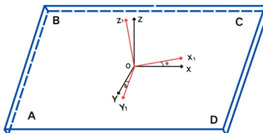
Fig. 1 – Schematic Diagram of the Rotation of the Chassis Coordinate System
