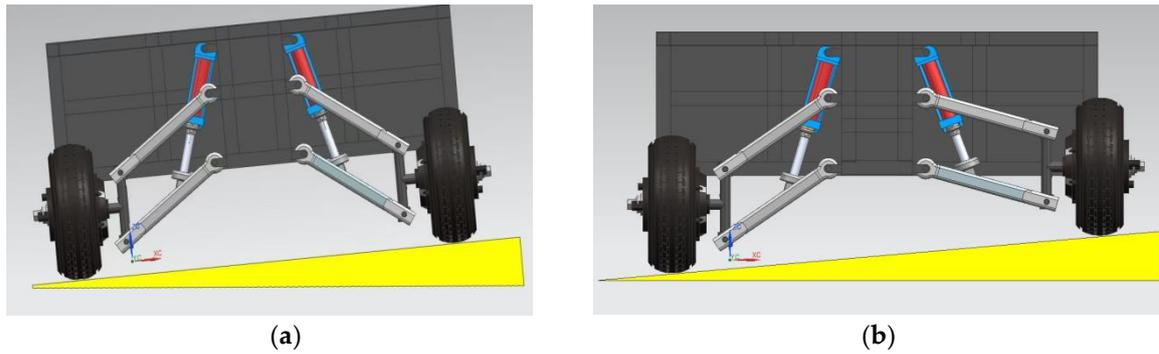
Schematic diagram of the leveling process in the transverse direction
