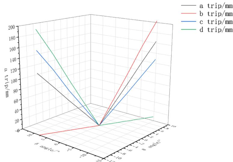
**Fig. 20 - Experiment Four: The Moving Amount of Each Hydraulic Cylinder Stroke under Different Inclination Angles**
