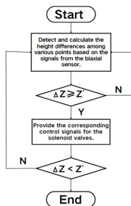
Fig. 11 - Control System Flowchart
