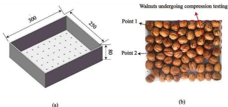
Fig. 4 – Arrangement of heat-treated walnut and fiber optic insertion point (a), shape and size of box (b) (mm)
