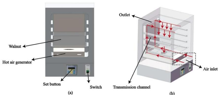
Fig. 5 – Schematic diagram of HA heating system
