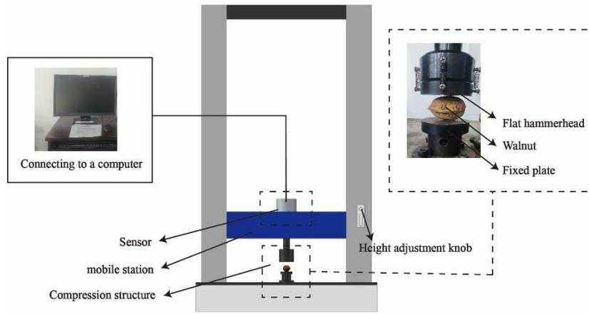
Fig. 1 – Schematic diagram of Mechanical Compression System
