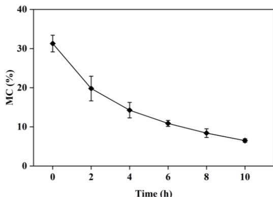
Fig. 6 –Drying curve of the sample (mean ± SD of two replicates)
