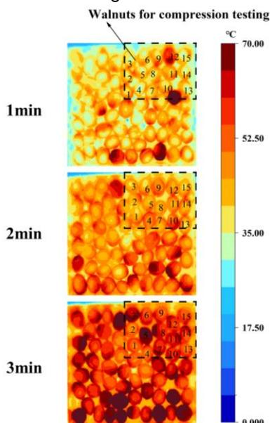
Fig. 10 – Temperature distribution of walnut surface after different RF treatment times
