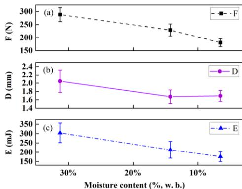
Fig. 7 –Samples rupture force-MC (a), rupture displacement-MC (b) and rupture energy-MC (c) (mean ± SD of five replicates)
