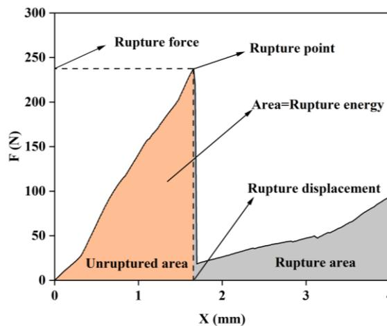
Fig. 2 – The classic force-displacement diagram of a walnut, showing the definitions of Rupture force (N), Rupture displacement (mm), and Rupture energy (mJ)
