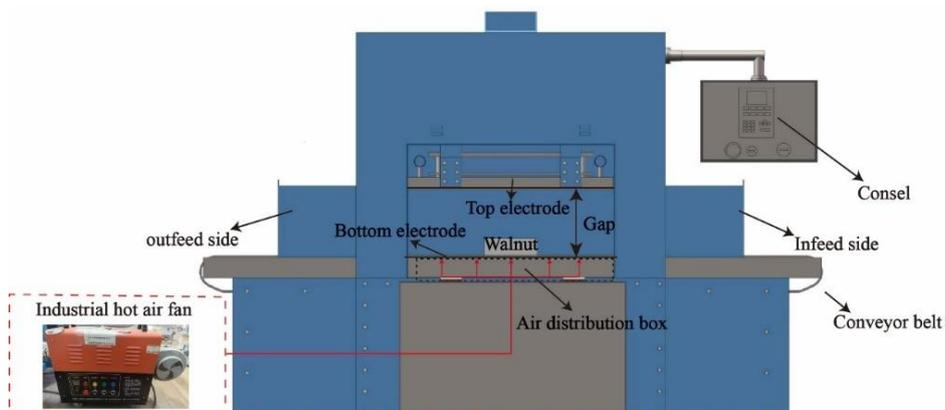
Fig. 3 – Schematic diagram of RF system
