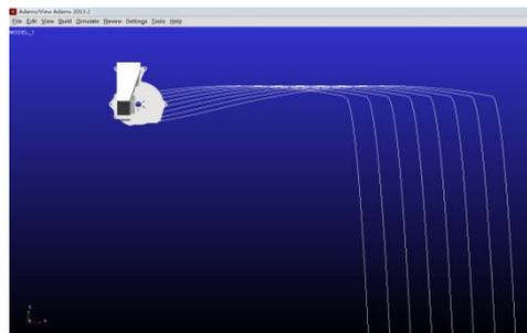
**Fig. 5 - Trajectory of seeds in operation 2**
