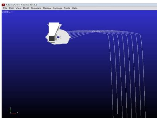
**Fig. 6 - Trajectory of seeds in operation 3**
