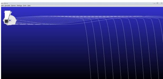
**Fig. 4 - The trajectories of seeds in operation 1**
