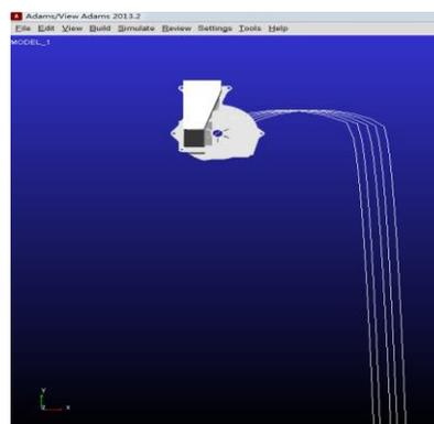
**Fig. 7 - Trajectory of seeds in operation 4**
