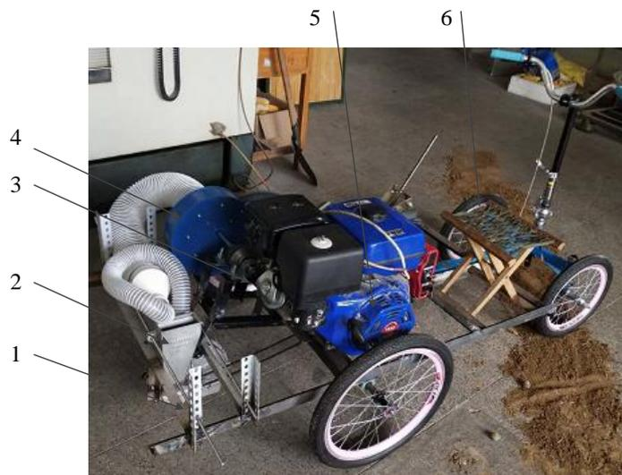
**Fig. 3 -Test bench of air-suction carrot seeder**
