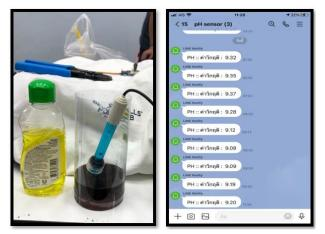
Fig. 4 - The result of system notification whenever the pH level fell below or exceeded the threshold
