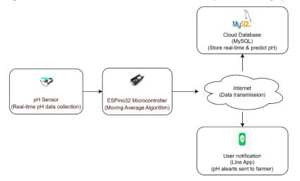
Fig. 1 - Infrastructure of the pH forecasting system for shrimp farms
