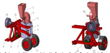
Fig. 1 - Schematic Diagram of the Air-Suction Garlic Sowing Unit Structure (1) Air suction garlic seeder; (2) Seeding shaft; (3) Chain; (4) Tensioning wheel; (5) Square bracket; (6) Ground wheel; (7) Profiling rod; (8) Pipe bracket; (9) Three-point suspension hanger; (10) Negative pressure fan; (11) Fixed bracket; (12) Belt pulley; (13) PTO device; (14) Negative pressure pipe
