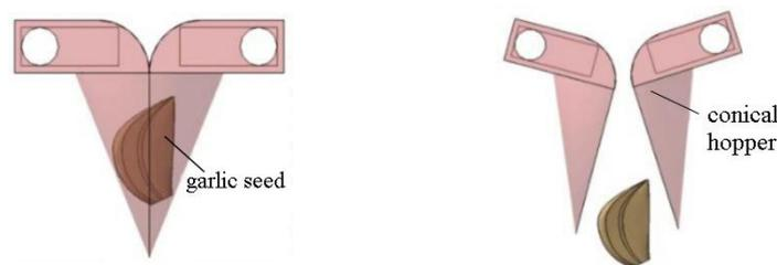
**Fig. 3 - Working process of conical hopper**
