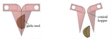
Fig. 3 - Working process of conical hopper
