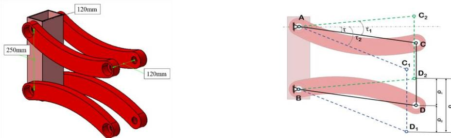
**Fig. 4 - Schematic Diagram and Dimensional Drawing of the Profiling Rod**
