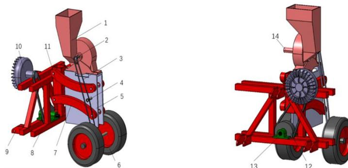
**Fig. 1 - Schematic Diagram of the Air-Suction Garlic Sowing Unit Structure**
