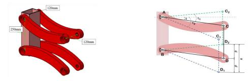
Fig. 4 - Schematic Diagram and Dimensional Drawing of the Profiling Rod
