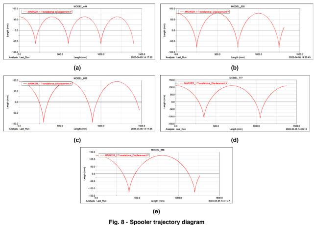
(a) 400 mm perimeter trajectory; (b) 500 mm perimeter trajectory; (c) 600 mm perimeter trajectory; (d) 700 mm perimeter trajectory; (e) 800 mm perimeter trajectory
