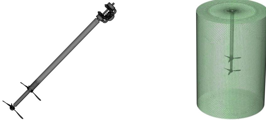
Fig. 4 -Agitator grid figure; flow field analysis grid diagram of fertilizer mixing tank
