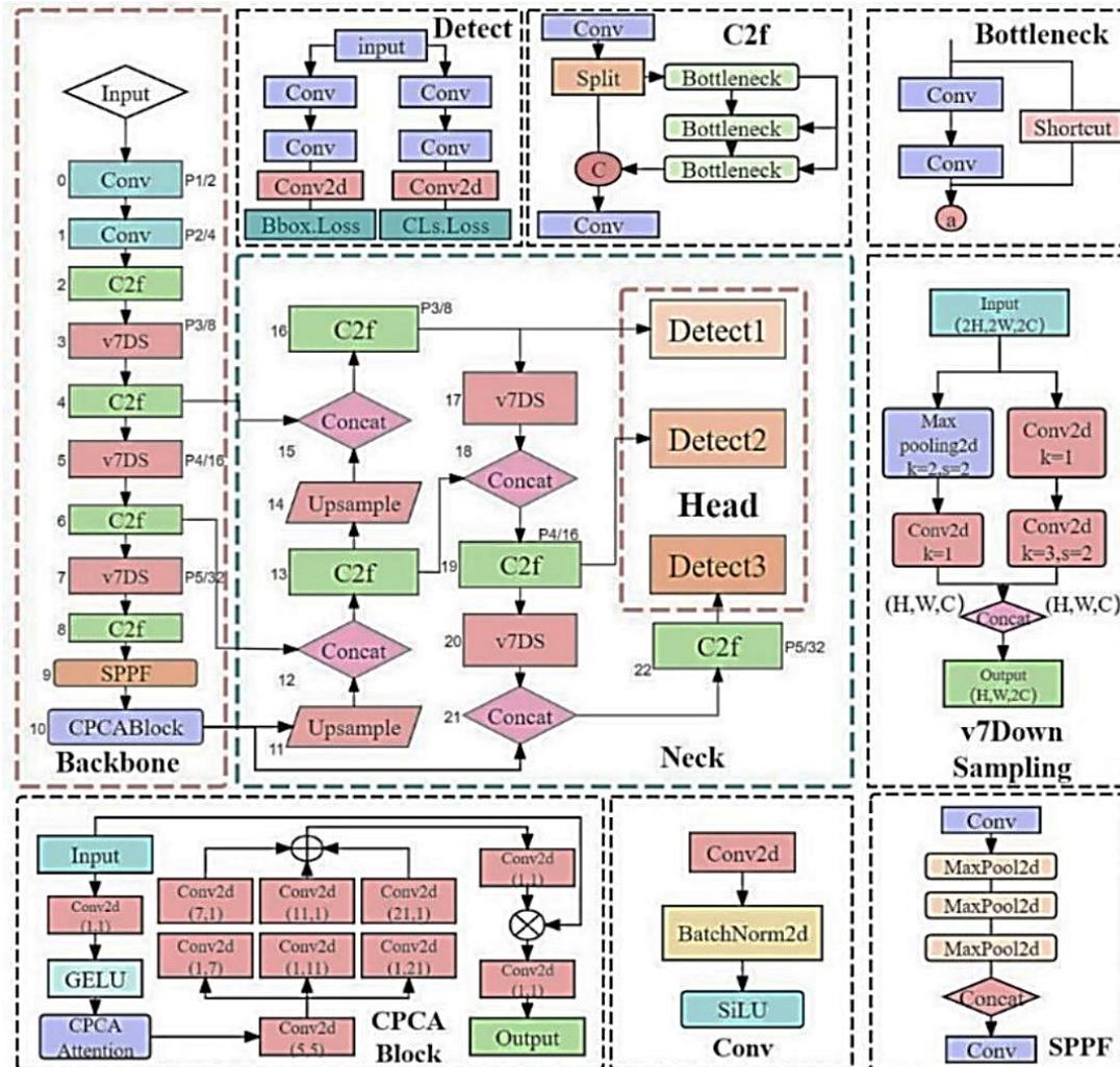
**Fig. 2 - Improved YOLOv8m model structure diagram**
