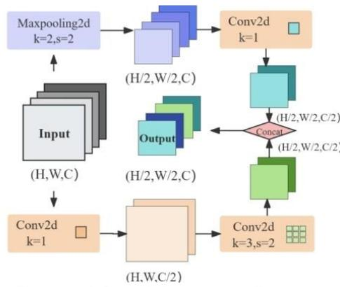
Fig. 3 -v7DS model structure diagram
