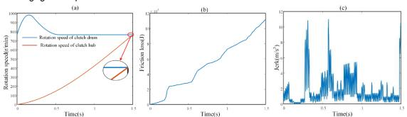
Fig.4 - Optimization results of clutch engagement process without considering terminal acceleration constraints
