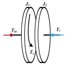
Fig. 2 - Model of clutch engagement process
