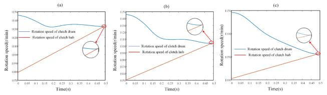
Fig. 7 - In hybrid systems, the clutch engages the optimal curve when the engine is involved
