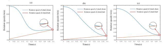
Fig. 6 - Optimal engagement curve of the clutch during the upshift process
