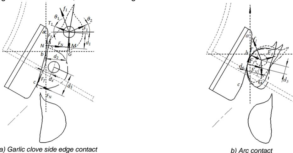
**Fig. 2 - Analysis of garlic clove contact guide cam process**
