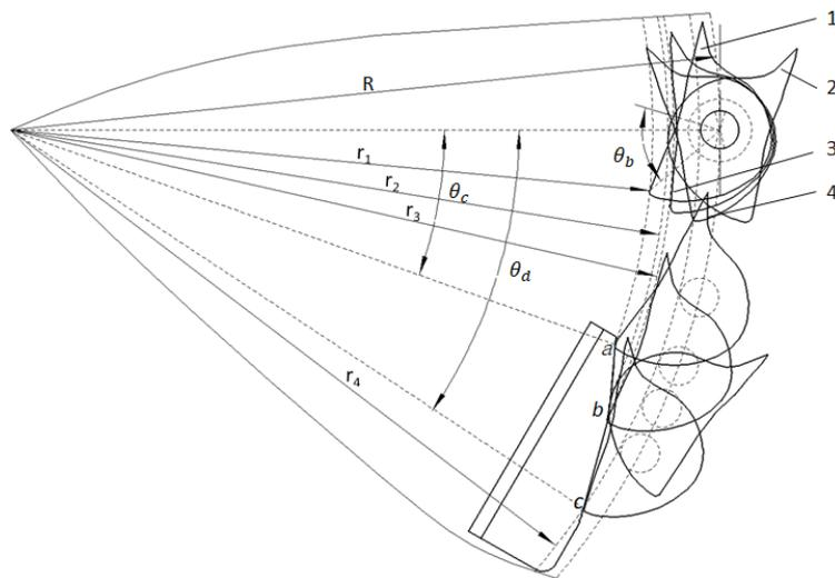
**Fig. 3 - Schematic diagram of the position where the garlic clove first contacts the guide cam**
