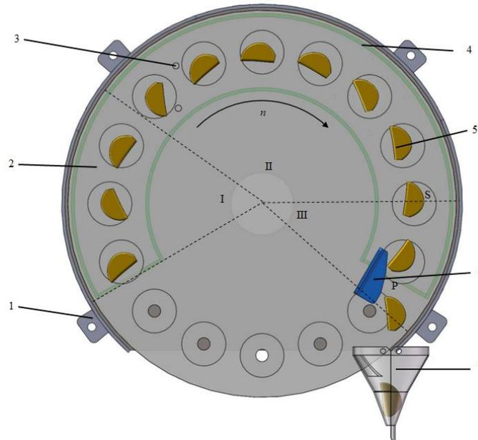
**Fig. 1 - Working principle diagram of a seed tray**
