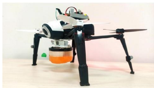
Fig. 12 - Spraying system reservoir developed
