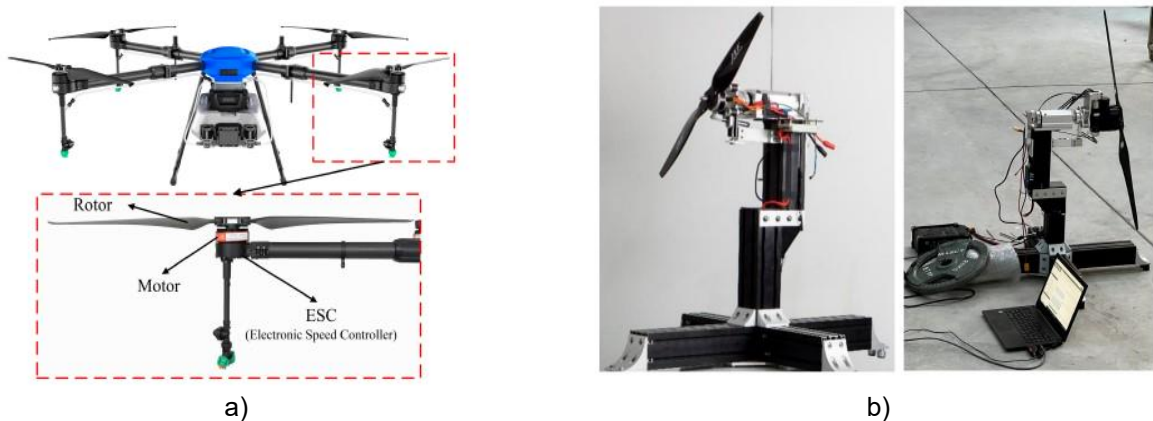
Fig. 13 – Rotor speed prediction model for multi-rotor unmanned aerial spraying systems
