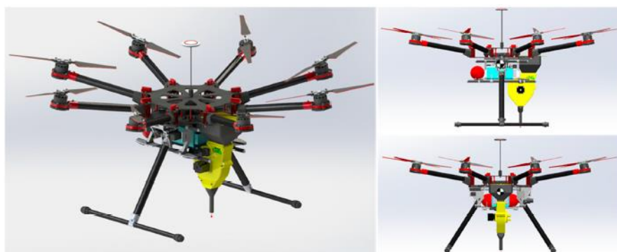
Fig. 11 - Seed metering device for aero sowing of forest pelleted seeds
