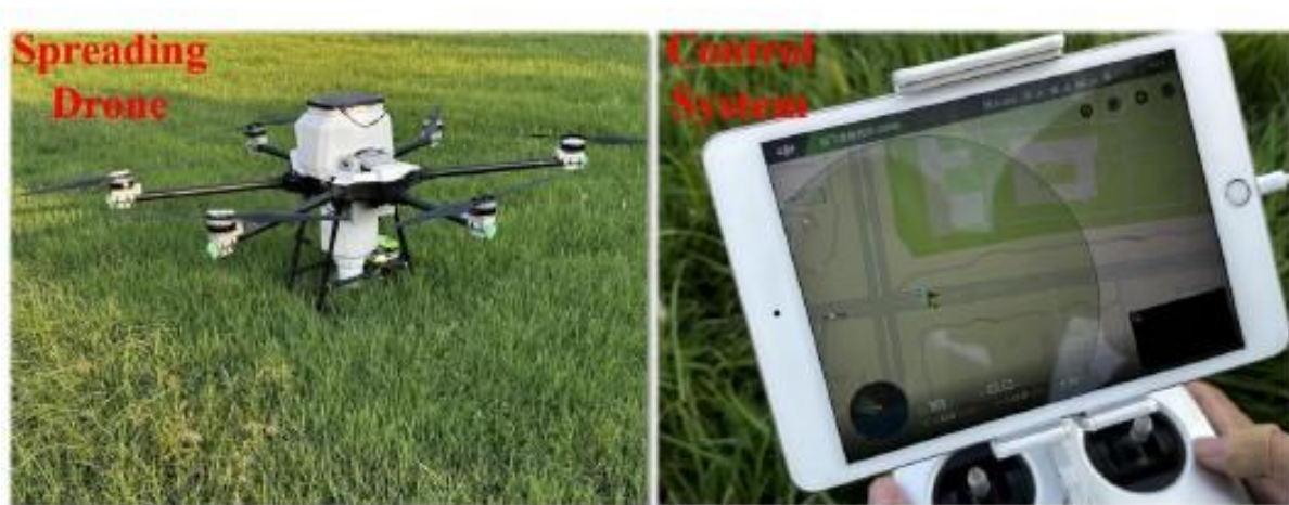
Fig. 7 - 6-rotor drone and spreading device controlled by DJI A3 system (Han et. al., 2024)
