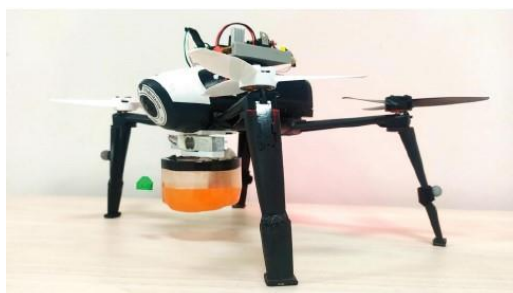
Fig. 12 - Spraying system reservoir developed
