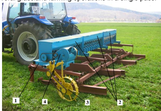
Fig. 3 - Grassland planer in aggregate with fertilizing equipment EF 3.75 type or sowing equipment ESR 3.75 type (Mocanu and Hermenean, 2008).
