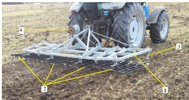
Fig. 5 - Harrow with rigid tines (Mocanu et al., 2022)
