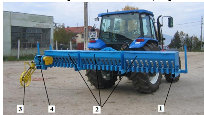
Fig. 2 - Fertilizing equipment EF 3.75 type; Sowing equipment ESR 3.75 type (Mocanu and Hermenean, 2008).
