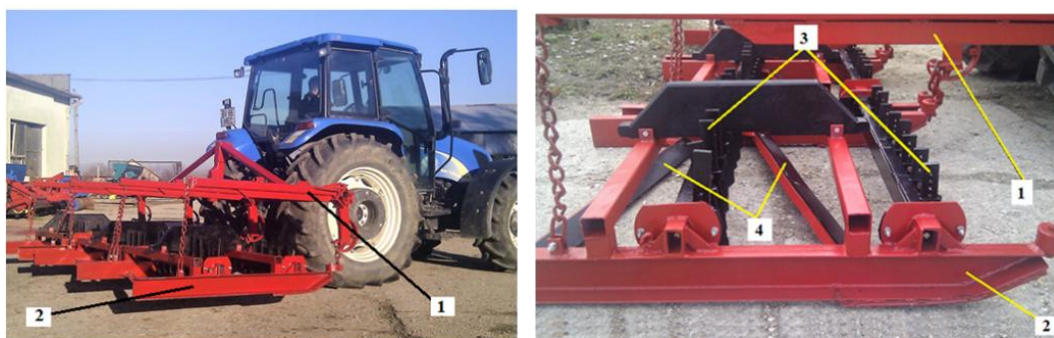
Fig. 4 - Grassland lever (Mocanu et al., 2022). a) aggregate view; b) detailed view of the work section
