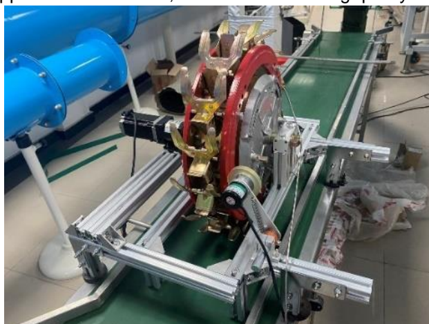
Fig. 8 - The seeding monitoring system test bench
