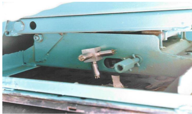
Fig. 6 - Accelerometers mounted on the harvester seat
