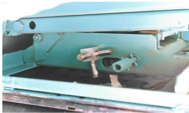
Fig. 6 - Accelerometers mounted on the harvester seat
