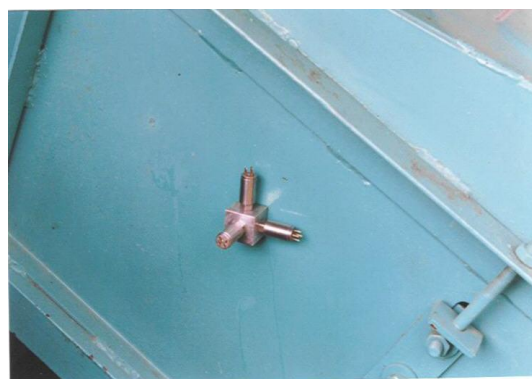
Fig. 5 - Accelerometers mounted on the harvester header
