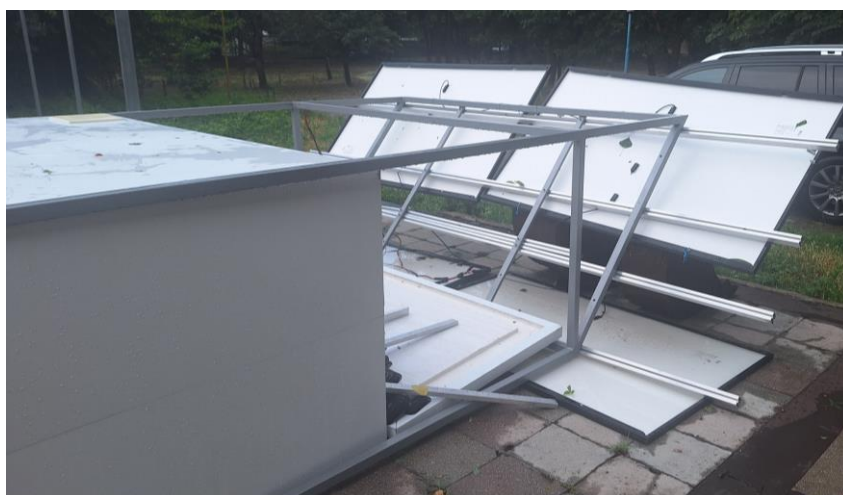
Fig. 4 – SVIEE vending machine overturned because of wind action
