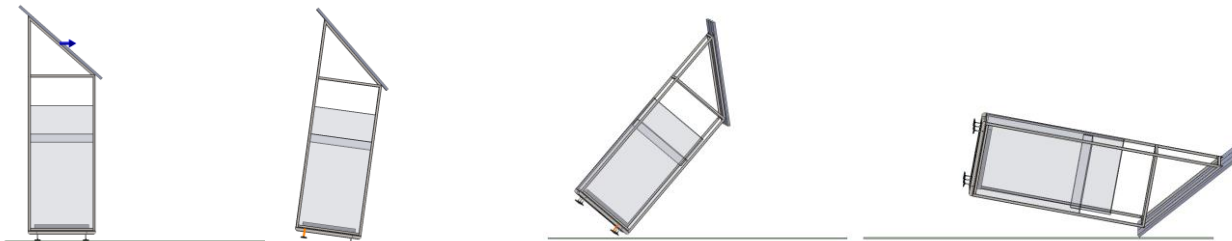
Fig. 9 – SolidWorks simulation of the loss of stability of SVIEE-R
