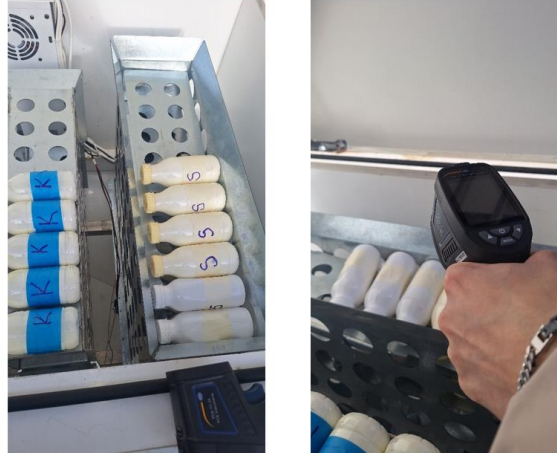
Fig. 6 – Loading the SVIEE-R with fermented dairy products. Temperature check with thermal camera.
