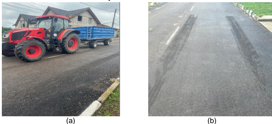
Fig. 2 – Object of study: a) Tractor Zetor Crystal HD 170; b) road surface and tire skid marks
