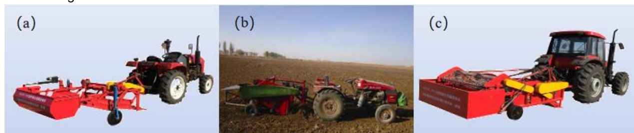
Fig. 9 - Screening type residual film recovery machine. (a) Shovel screen residual film recycling machine (Yan et al., 2017; You et al., 2017c); (b) Chain screen cultivator residue film recycling machine (Luo et al., 2018); (c) Net chain peanut residue film recycling machine (Xu et al., 2017)
