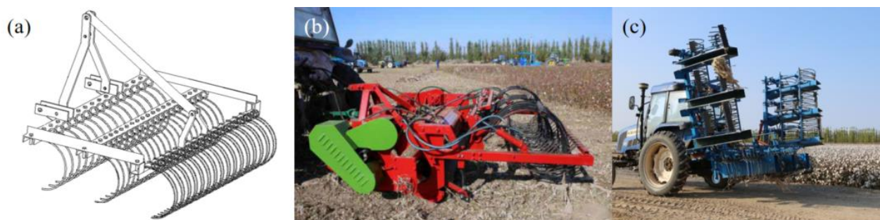
Fig. 5 - Representative tooth type residual film recovery machine
