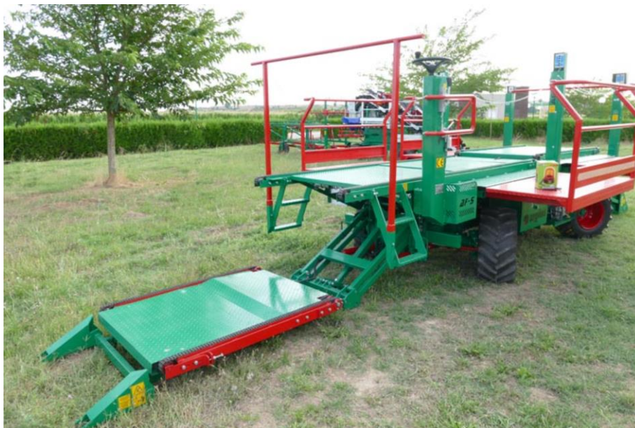
Fig. 2 - ARGILÉS AF-5, Machine for fruit picking, cutting, thinning, hail netting, etc. ( https://argiles.es/informacion-producto/af5/?lang=en )
