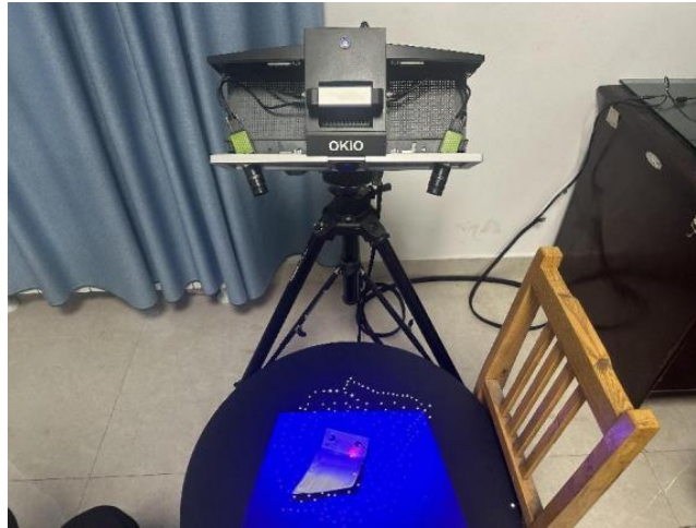
Fig. 4 – Scanning Process with COM1M-12 Type Grating 3D Scanner
