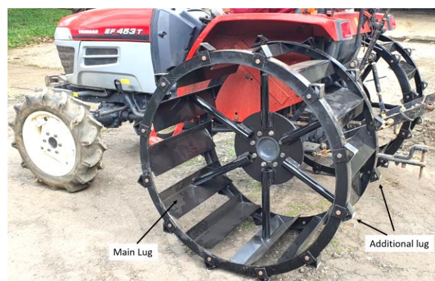
Fig. 2 - Cage wheel prototype installed on the tested tractor
