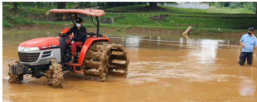
Fig. 5 – Setup and field measurement of turning diameter (TD)
