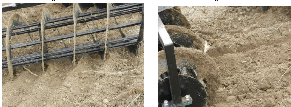
Fig. 2 – General view of the working surface of the screw harrow
