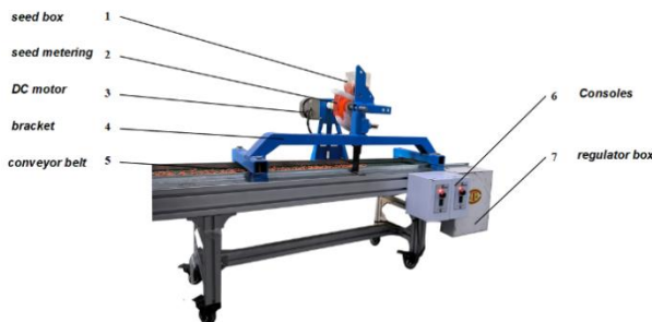
Fig. 11 - Coated wheat seed metering test device
